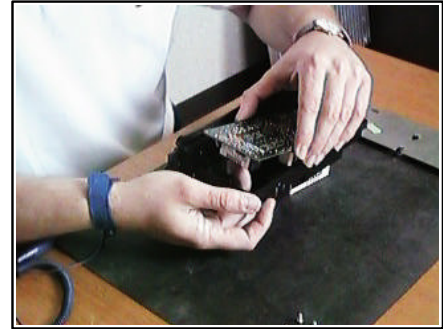
Figure 4. Remove PC board, push only on the plastic parts of the harness connectors
